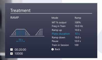
**Ramp mode.** Repetitive stimulation by trains with ramp up and down amplitude.
